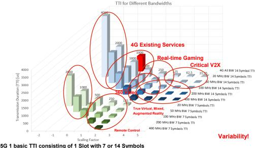
5G 1 basic TTI consisting of 1 Slot with 7 or 14 Symbols 4G 1 basic TTI has 2 slots with total of 14 Symbols
